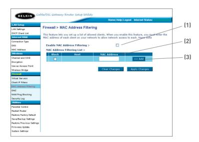
To enable this feature, select "Enable MAC Address Filtering" [1]. Next, enter the MAC address of each computer on your network by clicking in the space provided [2] and entering the MAC address of the computer you want to add to the list. Click "Add" [3], then "Apply Changes" to save the settings. To delete a MAC address from the list, simply click "Delete" next to the MAC address you wish to delete. Click "Apply Changes" to save the settings.
